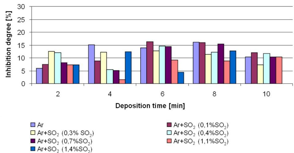
Fig. 2. Dependence of the degree of *Salmonella* bacteria development inhibition on the time of the film plasma modification in the Ar + (0-1.4%) SO<sub>2</sub> mixture.
