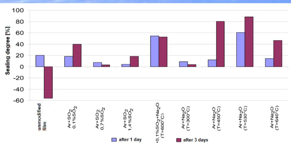
Fig. 5. Dependence of the sealing degree of the film towards water vapor on the type of modification; modification time of particular films = 6 min.
